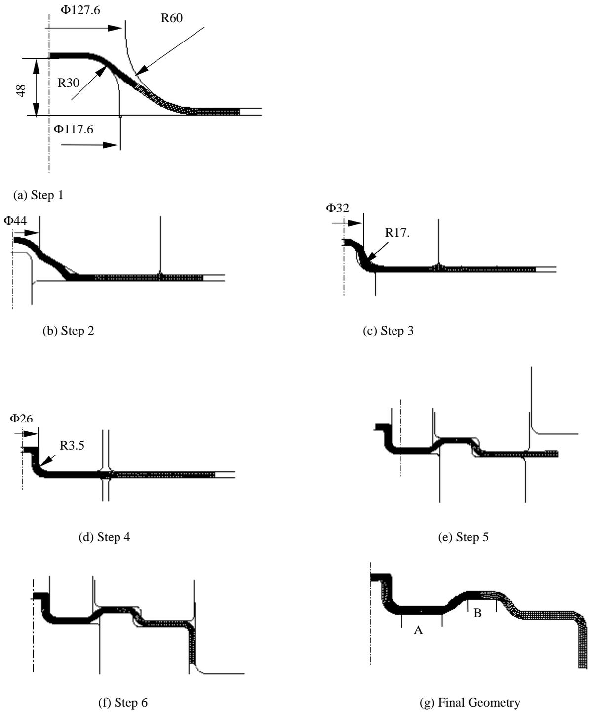
Fig.6 Deformed shapes of each drawing step in the new process
