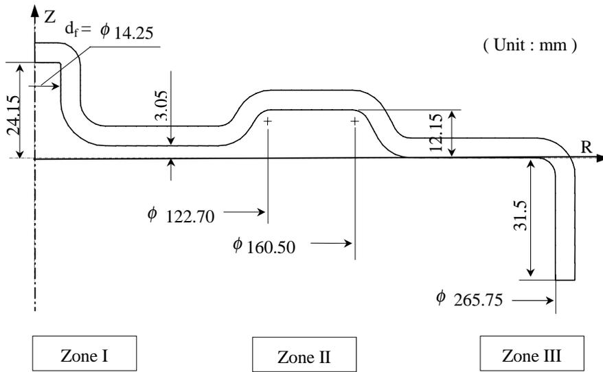
Fig.1 An automotive part of axisymmetric shape formed by multi-step drawing.
