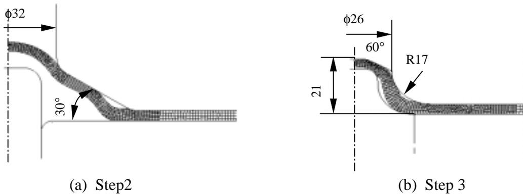
Fig. 4 New tooling geometries of steps 2 and 3.
