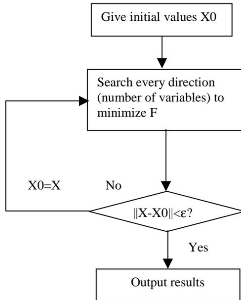
Fig.3 Optimization algorithm used in determining the tooling shape of Step 1.
