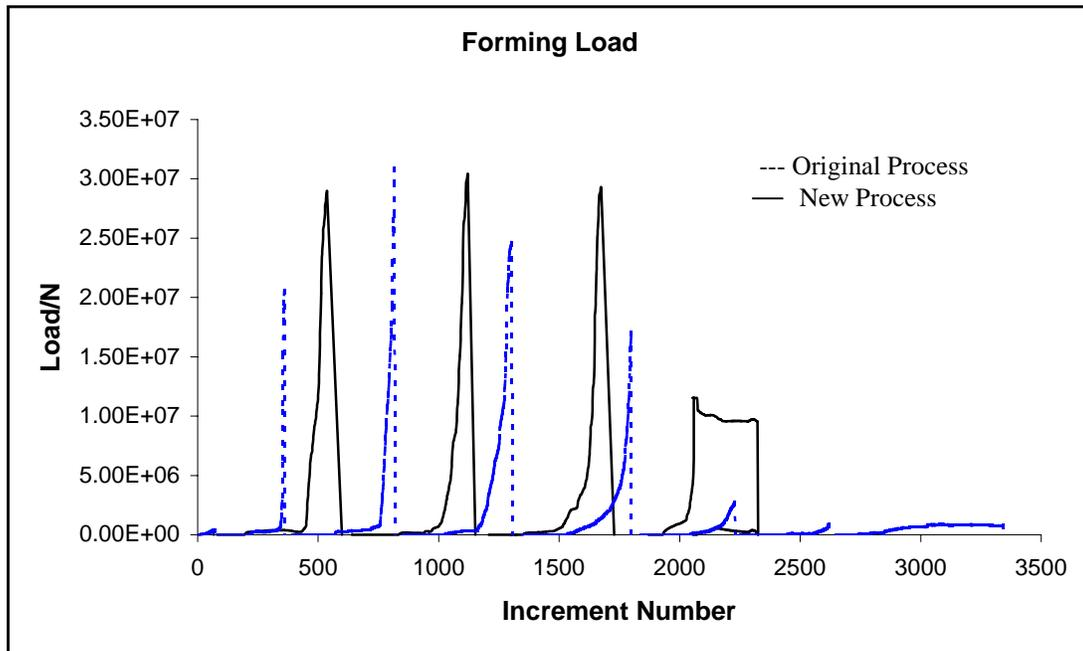
Figure 8 Forming Load of new & original processes
