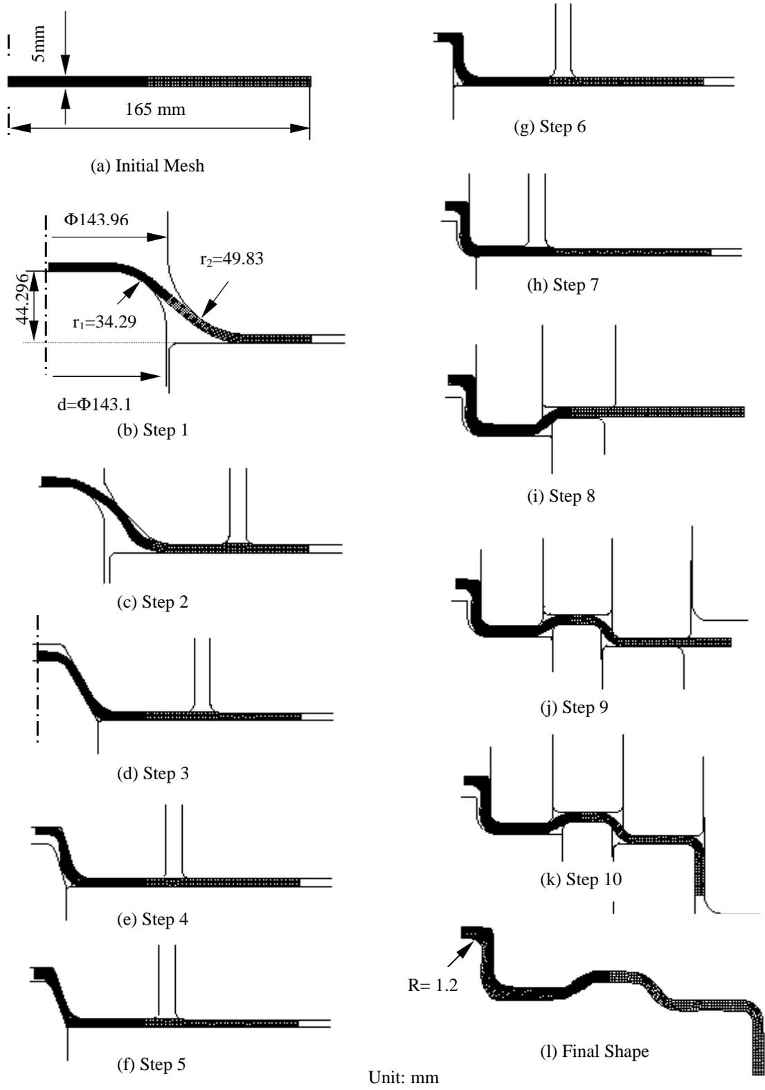
Fig.2 Initial geometry and deformed shapes for each drawing step in the original process.
